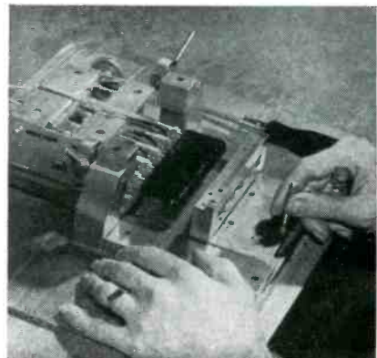
Tuner in position on fixture used to detect bent slides
