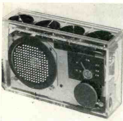
Four silicon solar cells on top of this portable radio, demonstrated by Hoffman Electronics, convert sun energy into electricity to operate the set.
