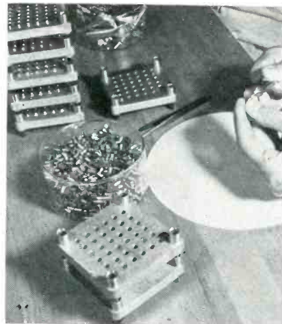
Squeezing potting compound from lead-foil tube into transistor can. Filled cans are stored in self-stacking metal trays as at upper left.
