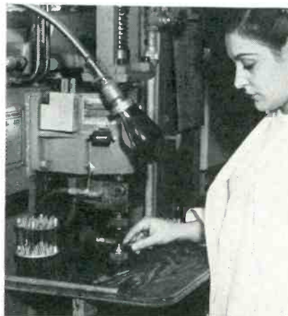
Placing transistor assembly in lower electrode of welder with tweezers. Welder output is indicated by counter, actuating arm of which is linked by string to move-able upper electrode of welder.
