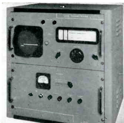
Reading on slide-rule dial corresponds to position of step on crt. left. Controllable inductors are in rectangular cans on r-f chassis at right in top view of receiver, center. Panoramic display, right, shows 1- \mu v and 1,000- \mu v signals separated by 500 kc
