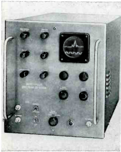
Control panel of multiple-pulse selector
