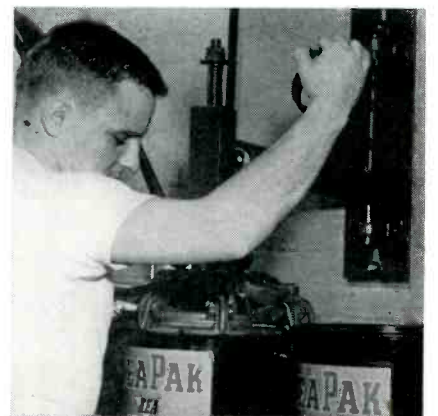
Setup for crimping covers on pails in one speedy operation at magnet wire plant
