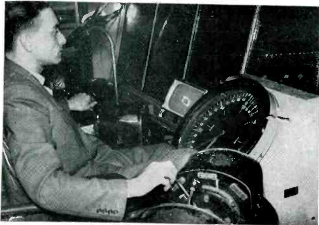
Operator at controls of slab rolling mill watches position of the ingot shown on the screen of tv monitor (left center) as seen by camera (upper right). Equipment on order from Marconi by Abbey
