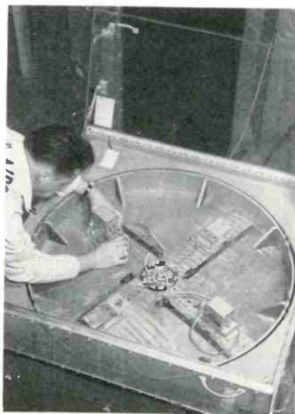
Installing component on centrifuge. Transparent plastic hinged covers are closed before starting drive motor under centrifuge
