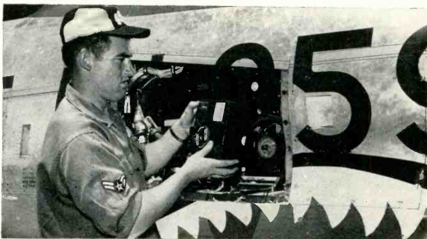
Magnetic tape magazine assembly and recorder, made by North American Aviation, is readied for flight as . . .
